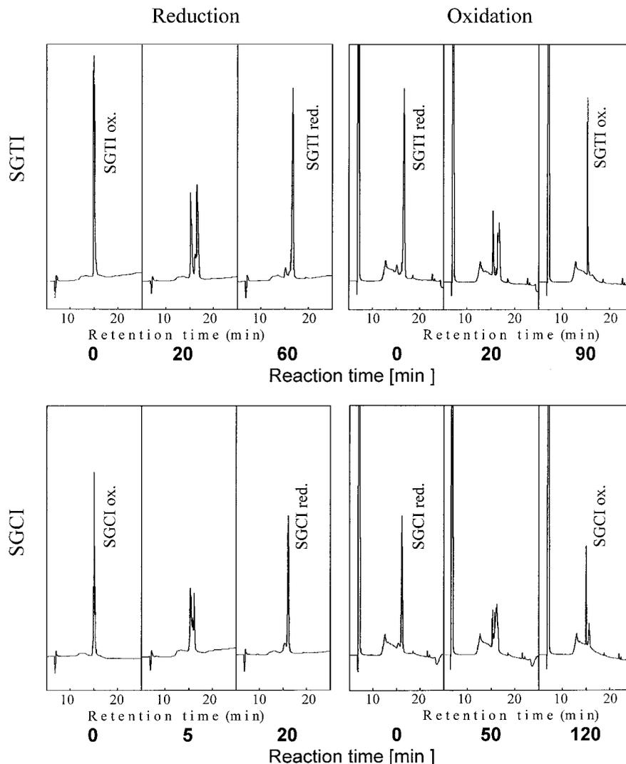
**FIG. 3.** HPLC profiles of samples withdrawn at indicated times from reduction (left) and oxidation (right) of SGTI (upper) and SGCI (lower). Conditions: flow rate, 1 ml/min; gradient, 0–100% B in 30 min (A, 0.1% TFA in water; B, 0.08% TFA in 80% acetonitrile/20% water). Detection at 220 nm. The middle part of each panel represents approximately 50% conversion.
