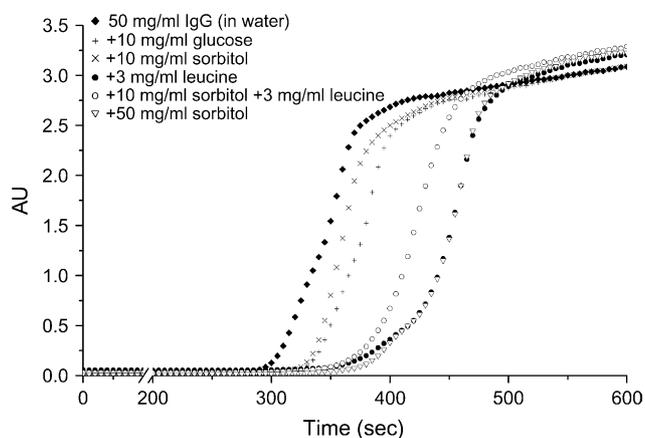
Fig. 6. Effect of excipients on the turbidity of IgG at 75 °C, 600 nm as a function of time. Aggregation process is delayed due to the stabilizers.
