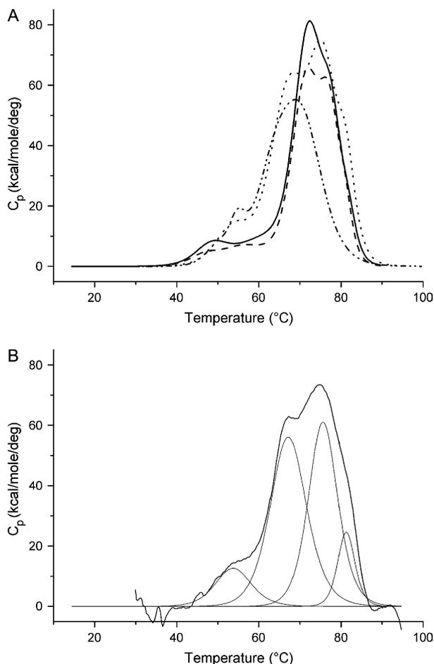
Fig. 2. (A) DSC thermograms of polyclonal IgG at pH 7.0 (solid line), pH 6.0 (dashed), pH 5.0 (dotted), pH 4.0 (dash-dot). (B) Deconvolution of the excess heat capacity functions of IgG at pH 5.0.
