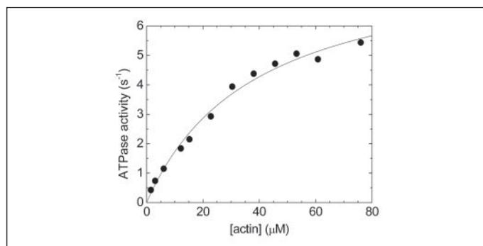
FIGURE 3. **Steady-state actin-activated ATPase activity of mVIIB-S1.** The ATPase activity of acto-mVIIB-S1 depended hyperbolically on actin concentration showing a  $V_{\text{max}}$  of  $8.4 \pm 0.6 \text{ s}^{-1}$  and a  $K_{\text{ATPase}}$  (actin concentration at half-maximal activation) of  $39 \pm 5 \mu\text{M}$ . Conditions:  $25^\circ\text{C}$ ,  $10 \text{ mM MOPS}$  (pH 7.0),  $2 \text{ mM MgCl}_2$ ,  $0.15 \text{ mM EGTA}$ ,  $1 \text{ mM ATP}$ ,  $10 \text{ mM KCl}$ .
